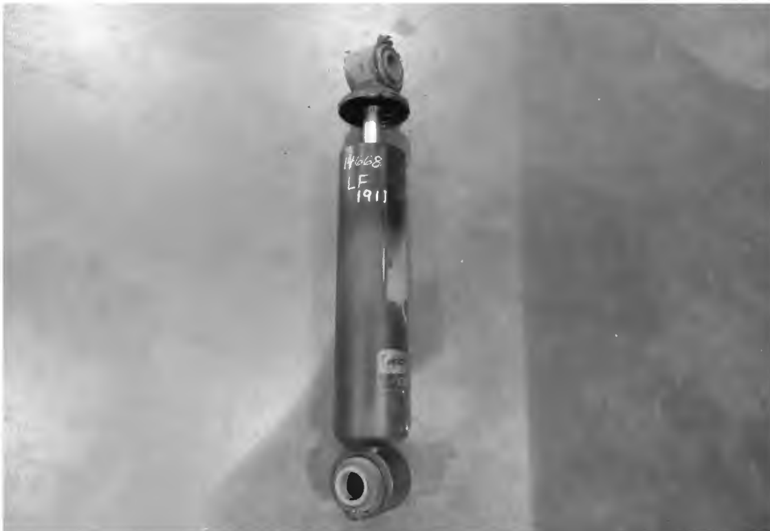
FRONT SHOCK LEAKING (11,491 TEST MILES)
