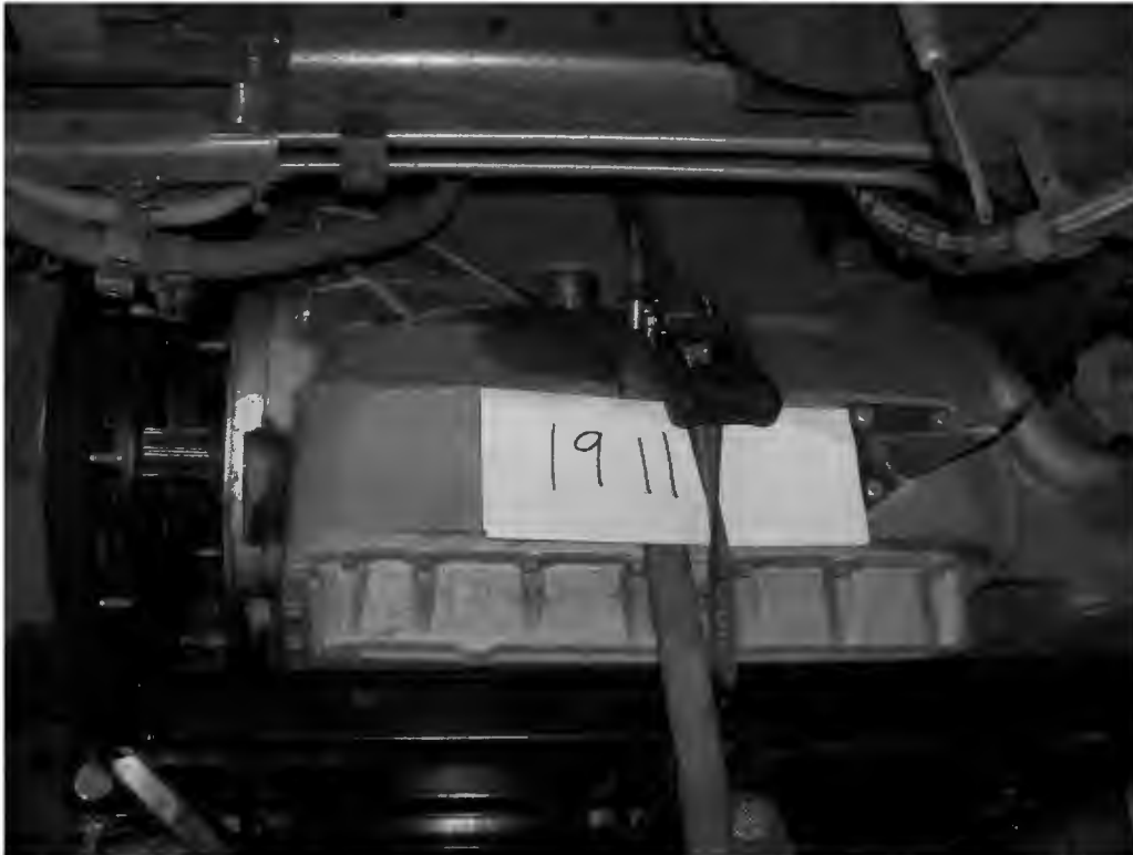
TRANSMISSION REMOVAL AND REPLACEMENT (6.00 LABOR HOURS)
