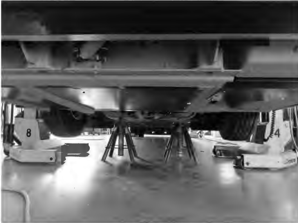
JACK STANDS IN PLACE-FRONT OF BUS
