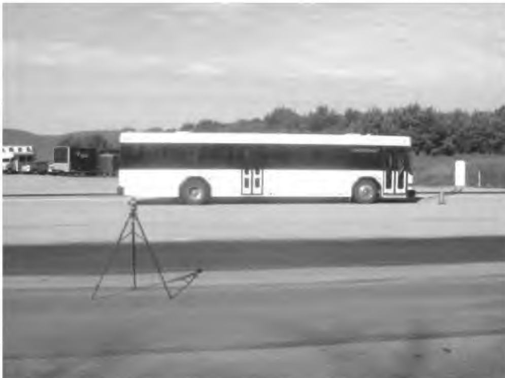
TEST BUS UNDERGOING EXTERIOR NOISE TESTING
