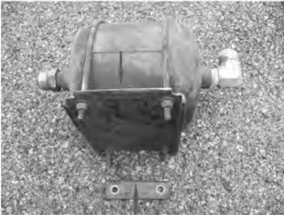
FAILED AIR TANK MOUNTING BRACKET (8,074 TEST MILES)
