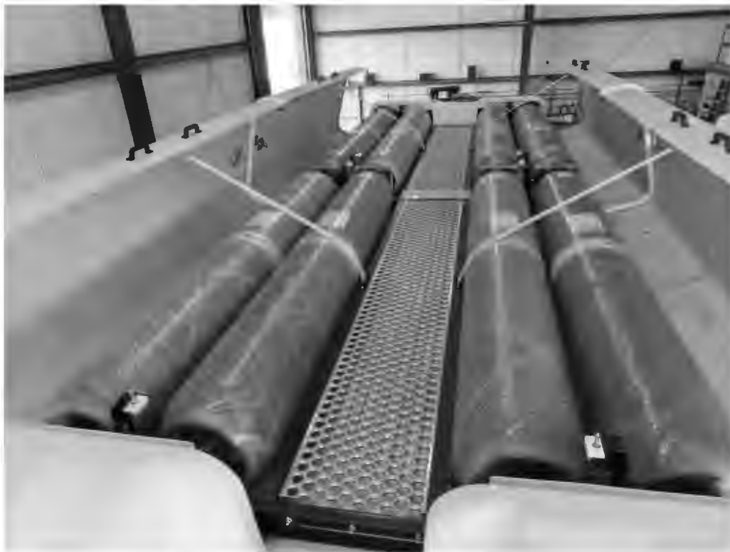
ROOFTOP CNG TANKS
