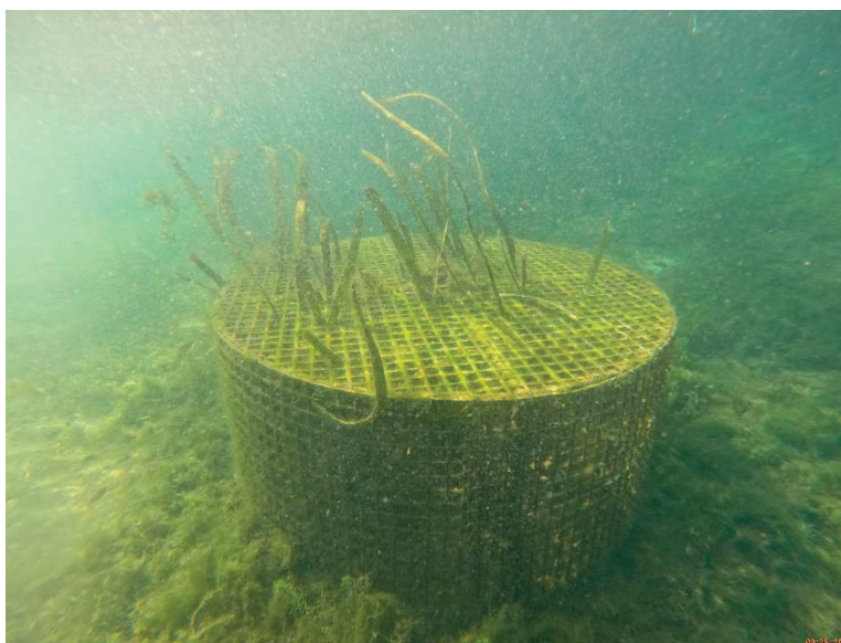
Figure 1. Example of biofouling prior to removal.
