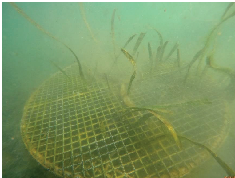
Figure 3. Example of GrowSAV Device after biofouling removal.
