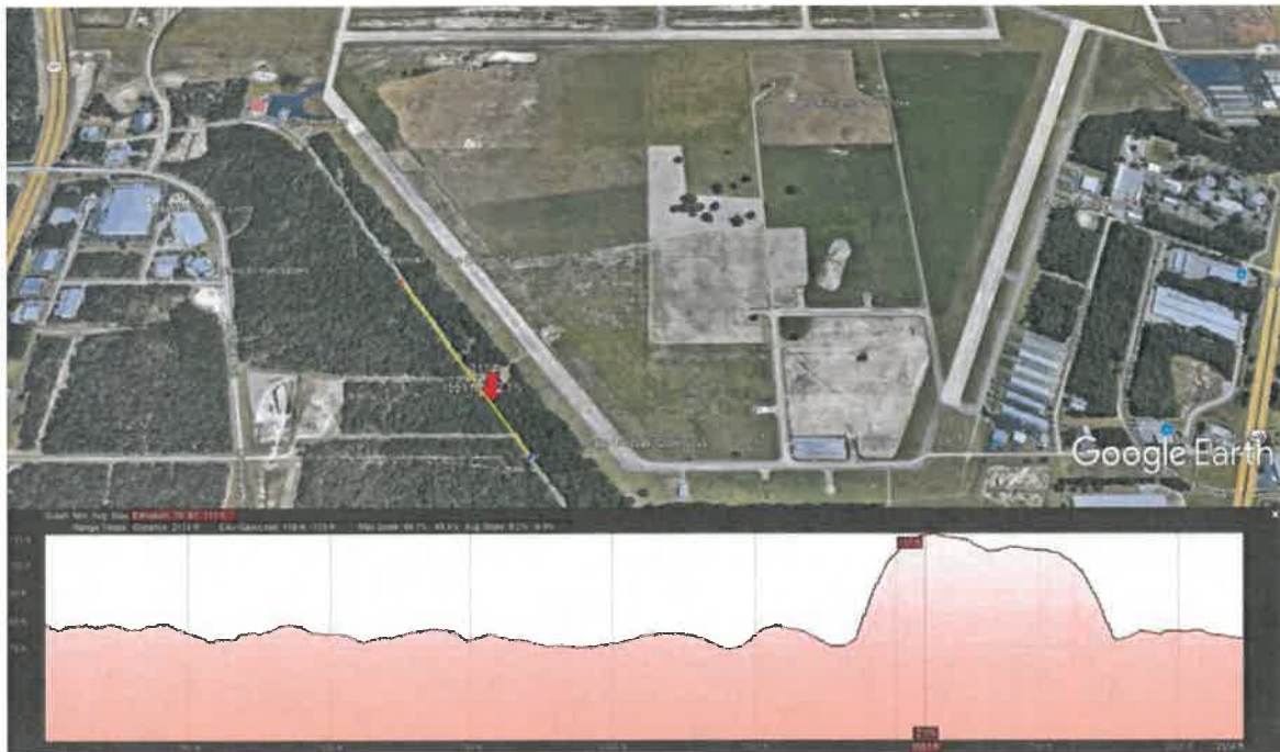
Figure 5-2: Ground Elevation Profile along the New Road Connecting Telecom Dr. and Airport Service Rd and Approximate ARV Placement (Red Arrow)
