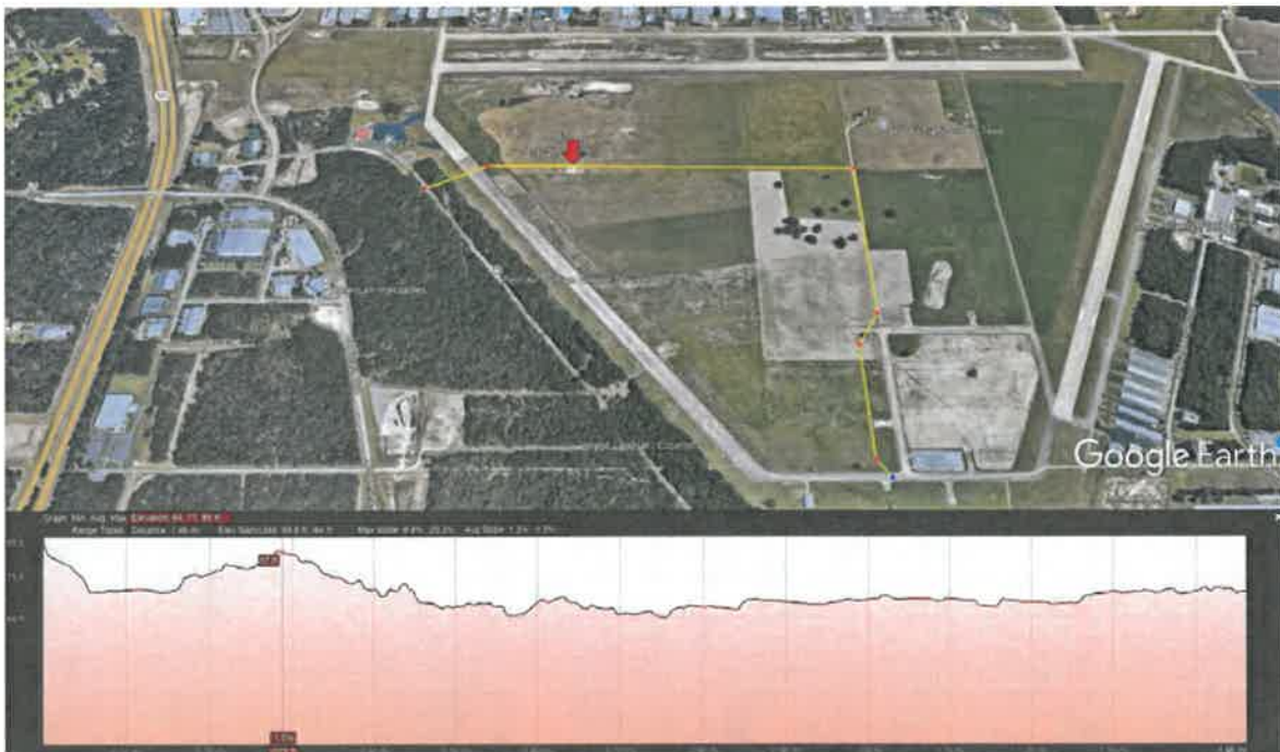
Figure 5-3: Ground Elevation Profile along the New Road Going East to West across the BKV Infield area and Approximate ARV Placement (Red Arrow)
