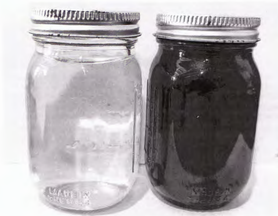
Figure 4-2. Raw Leachate (Right) and Treated Permeate (Left) at New River Regional Landfill ROBOX System.
