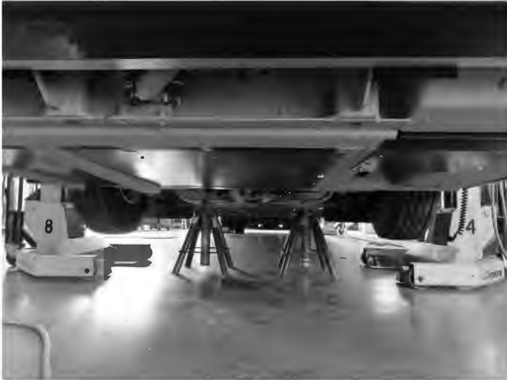
JACK STANDS IN PLACE-FRONT OF BUS
