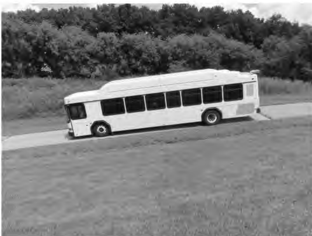
PARKING BRAKE TEST PARKING BRAKE HELD FOR 5 MINUTES IN BOTH 20% UP AND 20% DOWN POSITIONS
