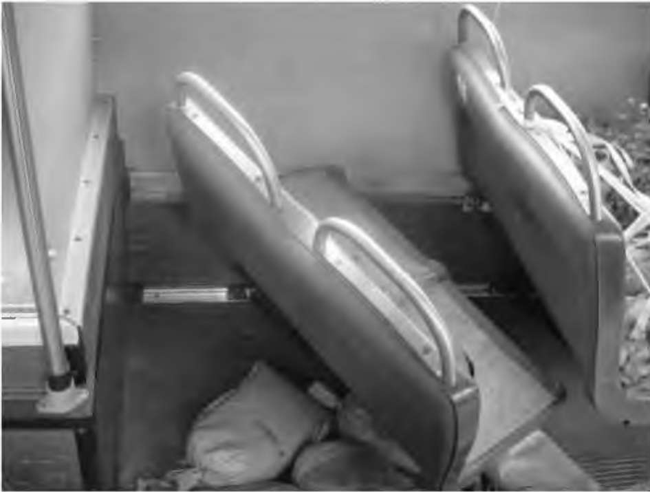
BROKEN SEAT FRAME (5,500 TEST MILES)
