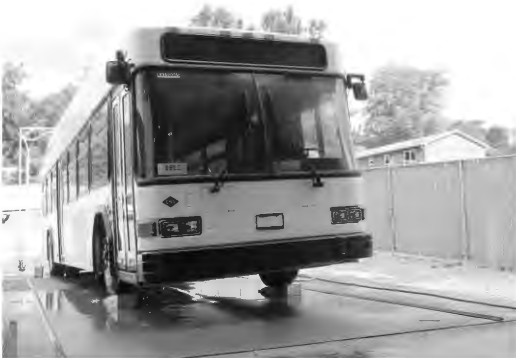
RIGHT REAR WHEELS SIX INCHES LOWER
