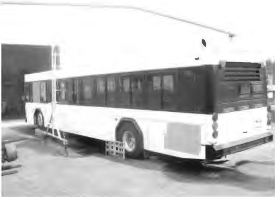
RIGHT REAR WHEEL SIX INCHES LOWER
