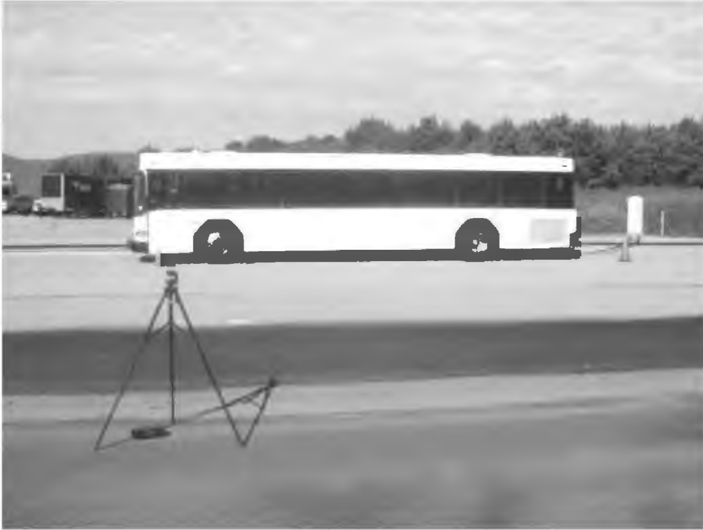
TEST BUS UNDERGOING EXTERIOR NOISE TESTING
