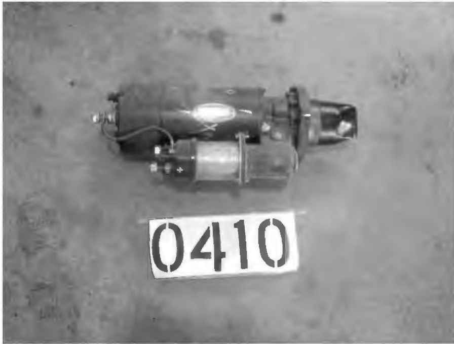
STARTER REMOVAL AND REPLACEMENT (0.75 MAN HOURS)
