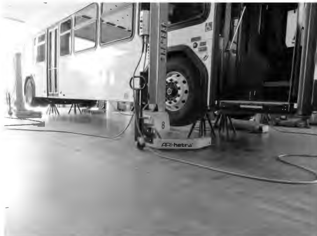
JACK STANDS IN PLACE-FRONT AND REAR OF BUS
