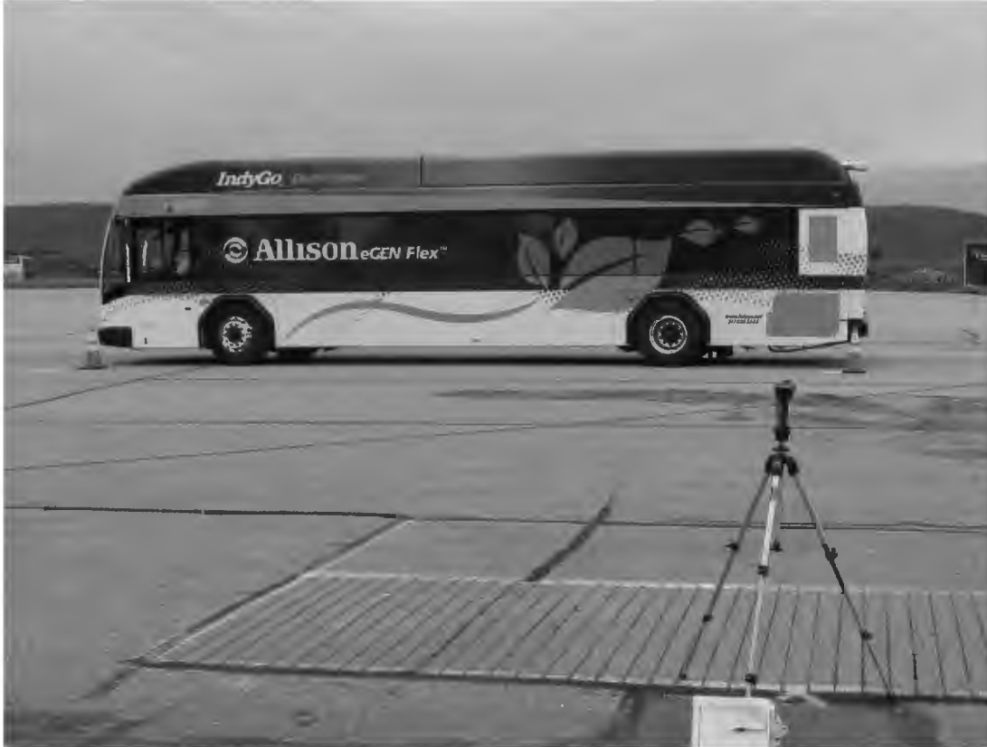
TEST BUS UNDERGOING EXTERIOR NOISE TESTING
