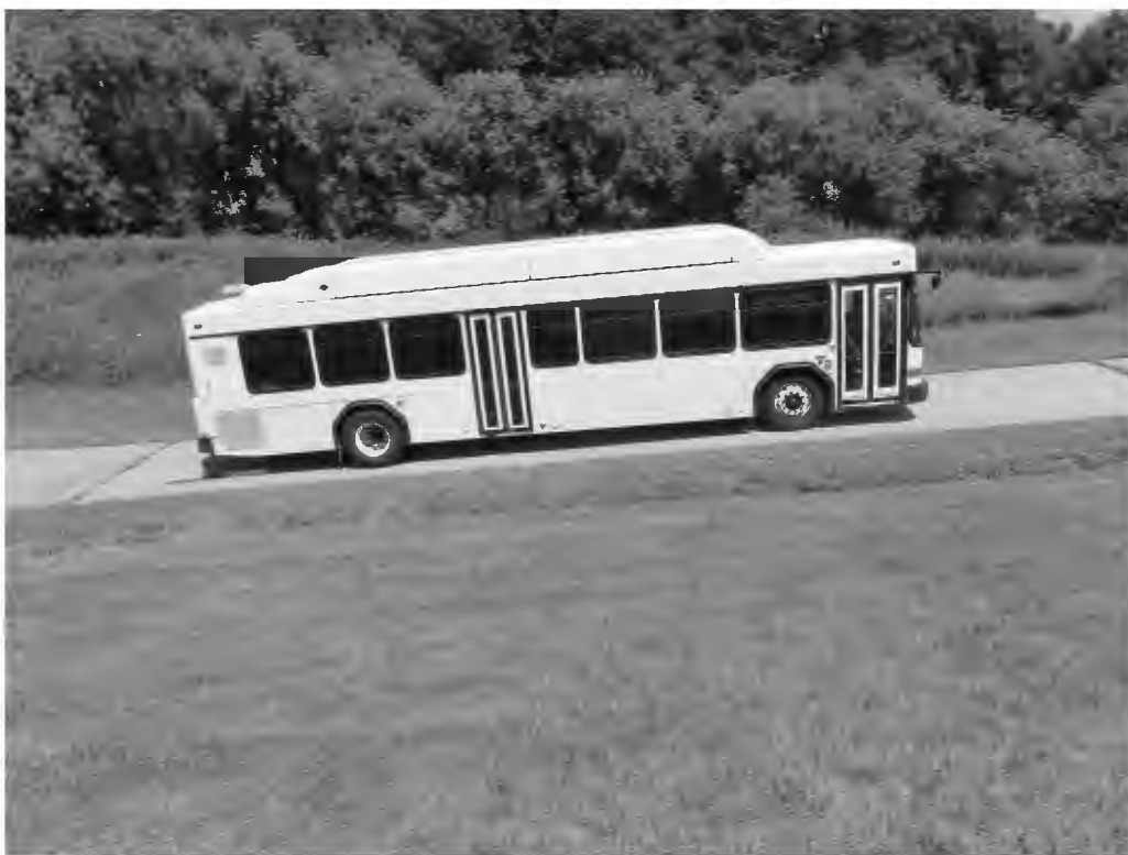
PARKING BRAKE TEST PARKING BRAKE HELD FOR 5 MINUTES IN BOTH 20% UP AND 20% DOWN POSITIONS
