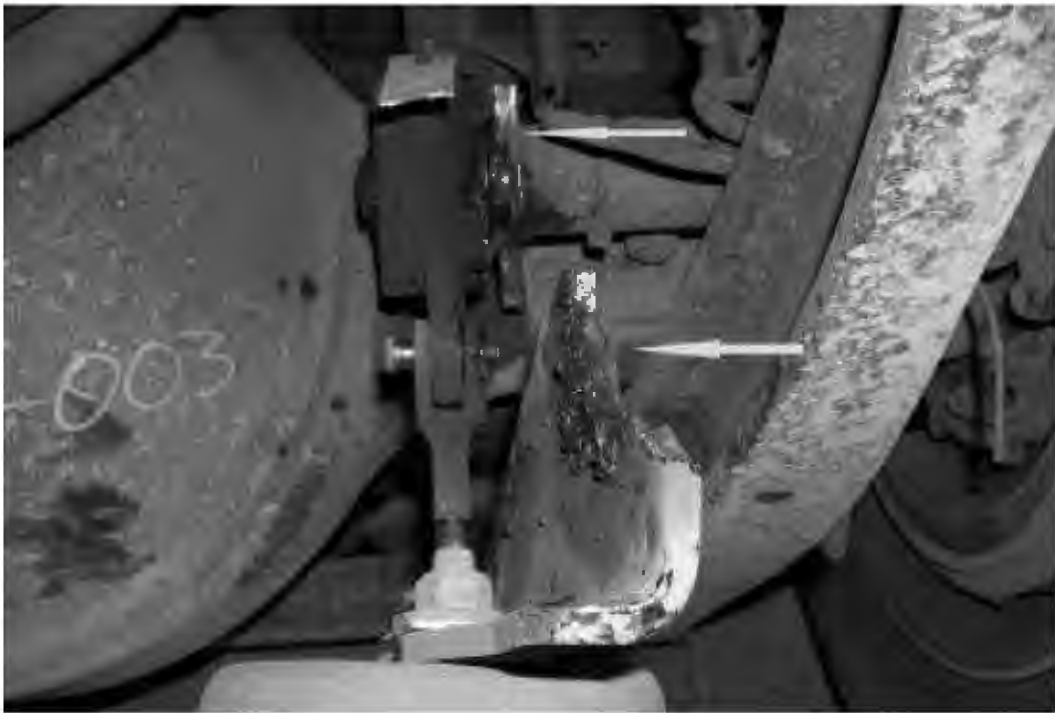
BROKEN LEFT REAR BRAKE CHAMBER BRACKET (5,451 TEST MILES)
