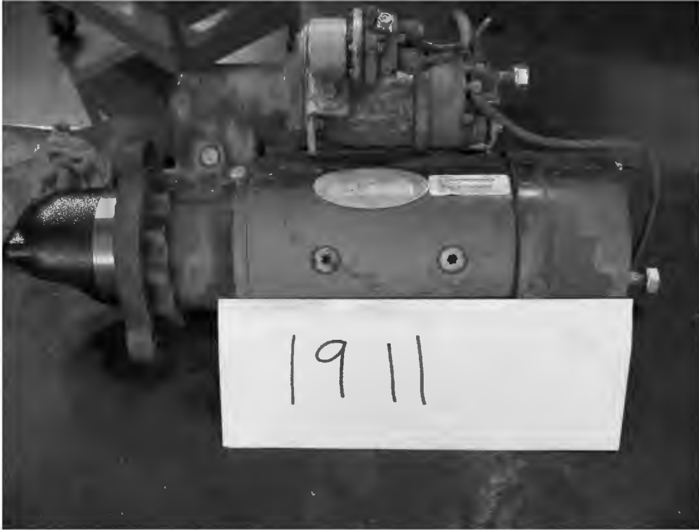
STARTER REMOVAL AND REPLACEMENT (1.00 LABOR HOUR)
