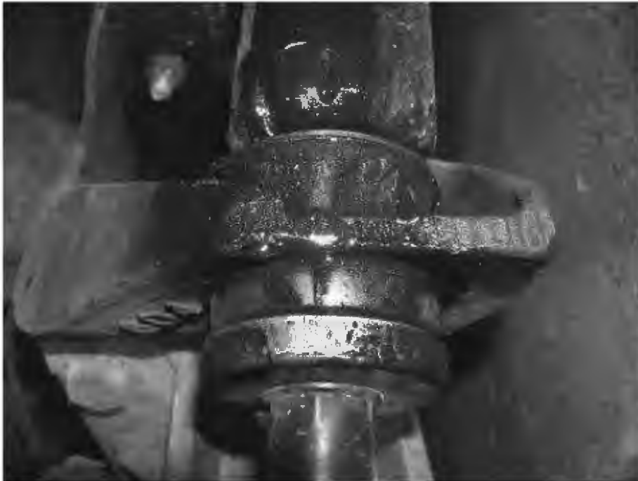
FRONT SHOCK LEAKING OIL (4,379 TEST MILES)
