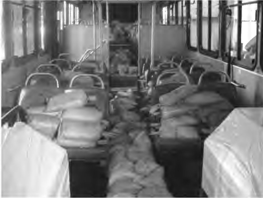
BUS LOADED TO 2.5 TIMES GVL (28,125 LBS)
