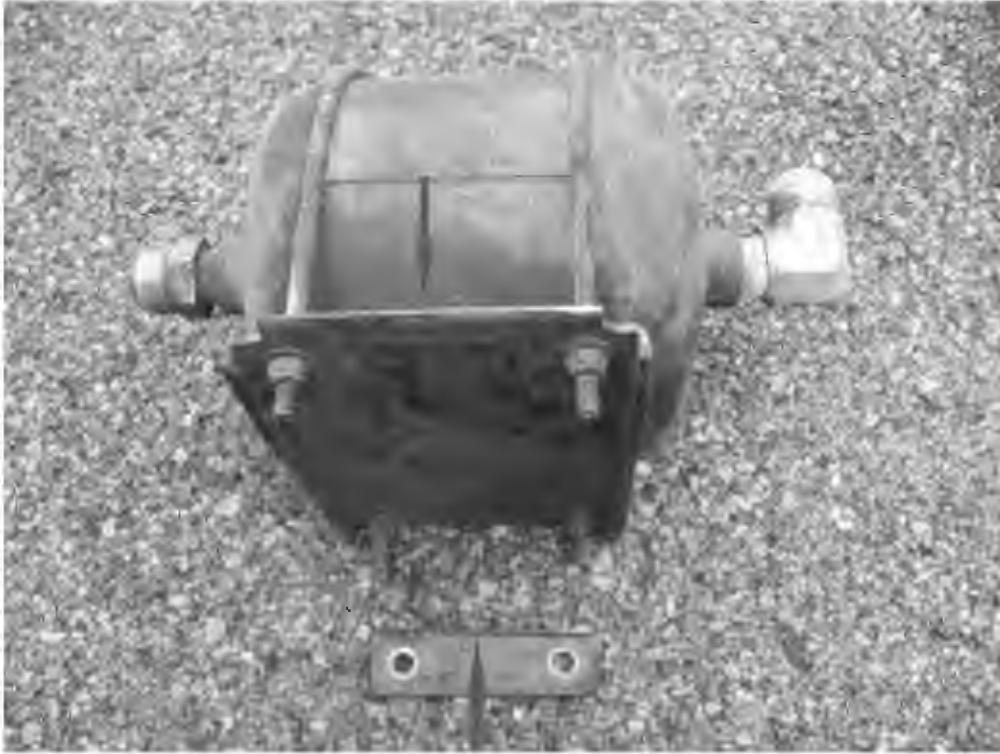
FAILED AIR TANK MOUNTING BRACKET (8,074 TEST MILES)
