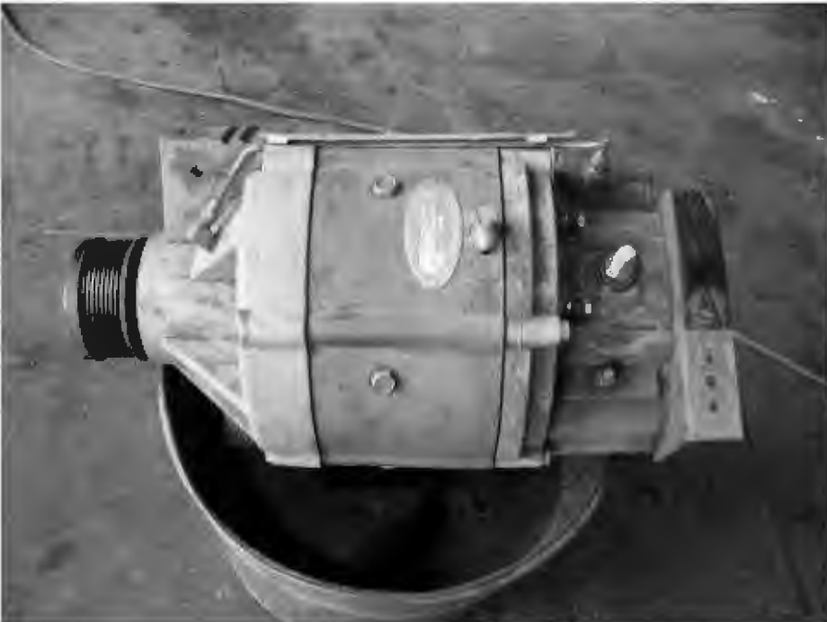
FAILED ALTERNATOR (4,730 TEST MILES)
