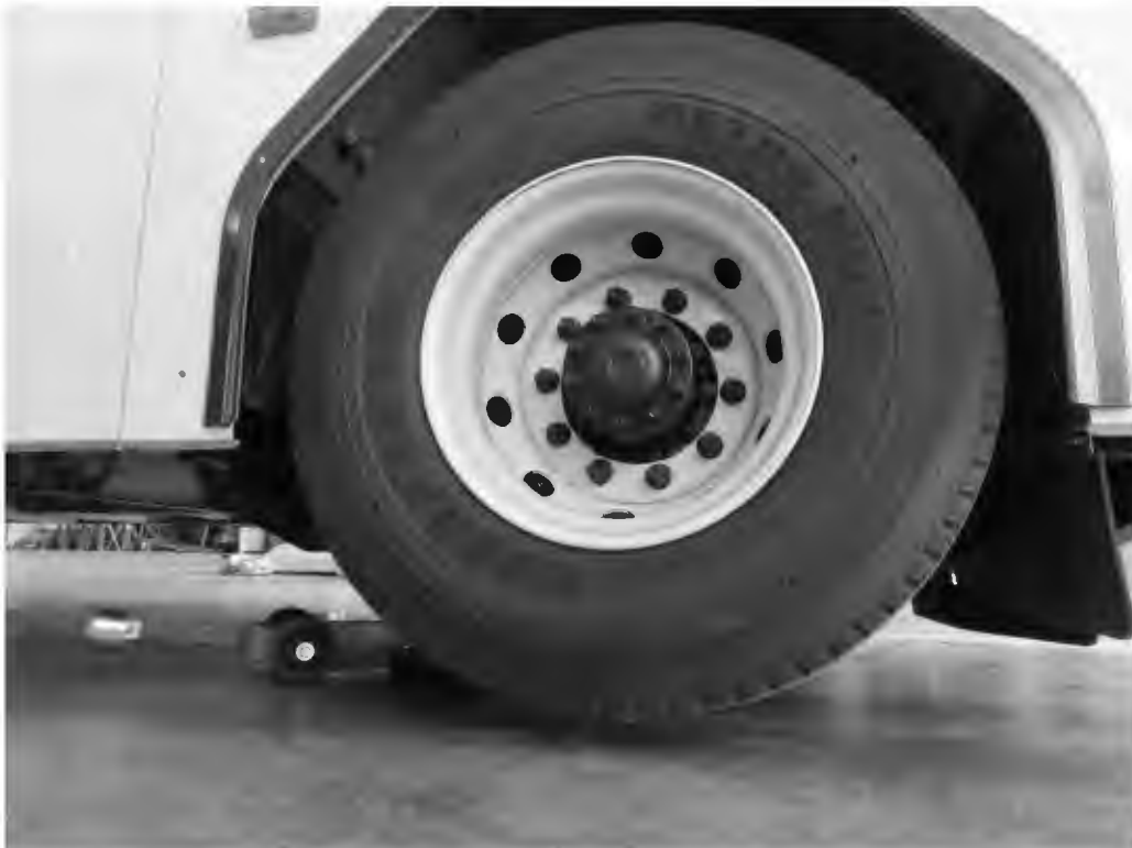
JACK IN PLACE-REAR
