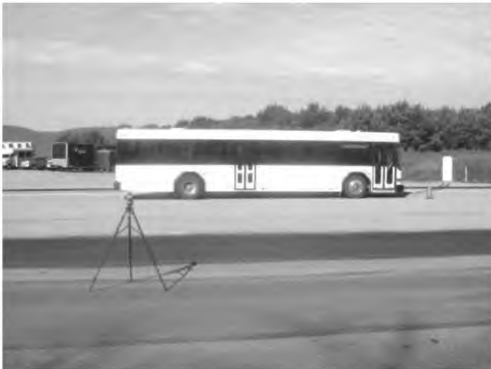
TEST BUS UNDERGOING EXTERIOR NOISE TESTING
