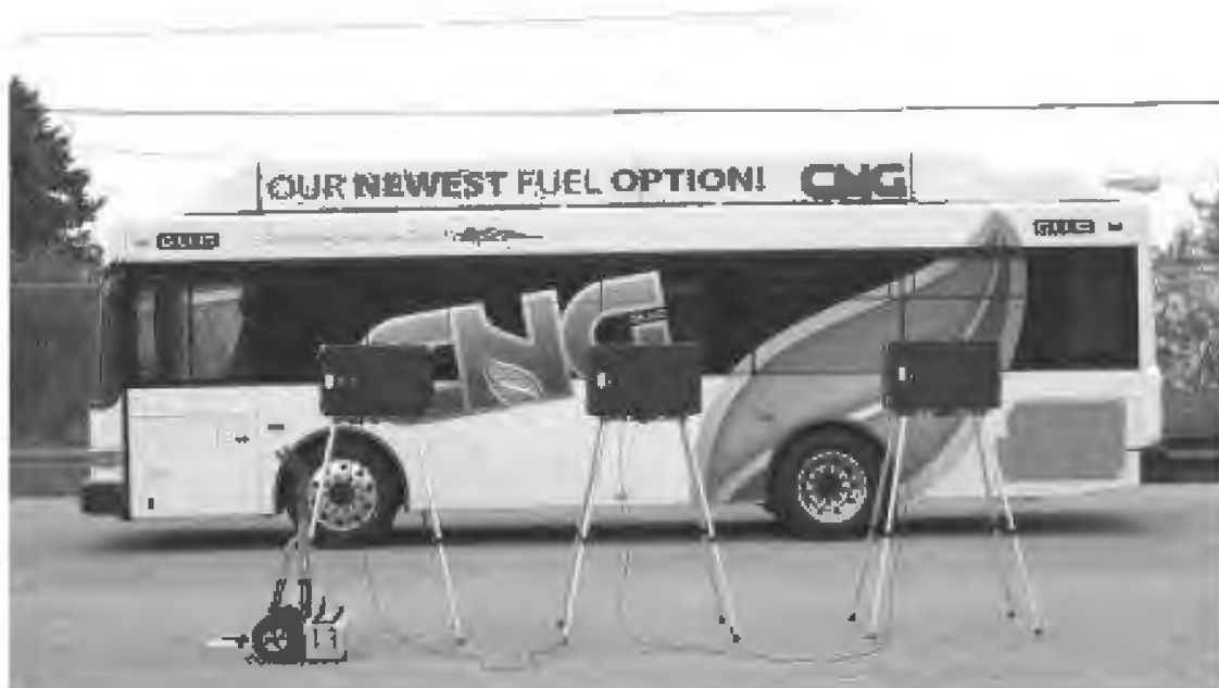
TEST BUS SET-UP FOR 80 dB(A) INTERIOR NOISE TEST
