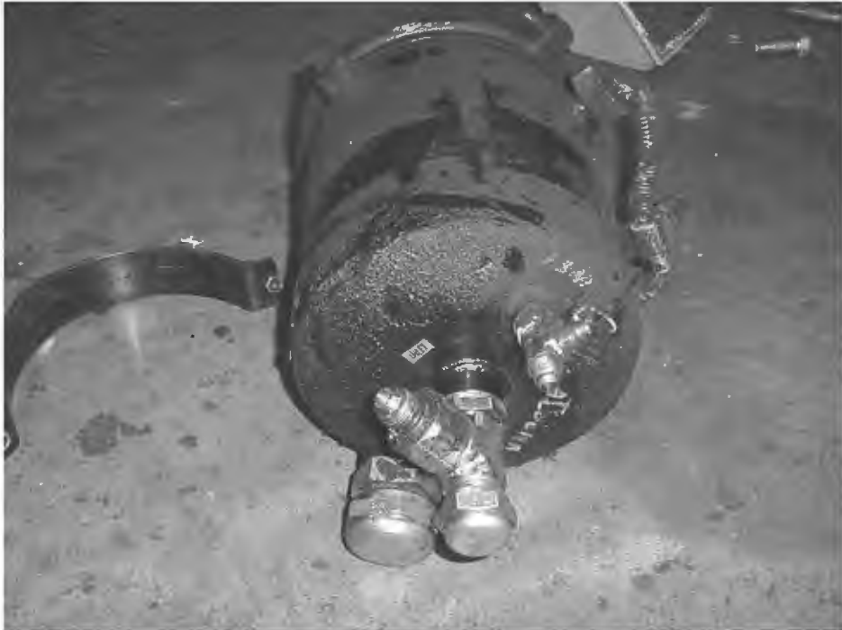
CRACKED HYDRAULIC RESERVOIR (12,487 TEST MILES)
