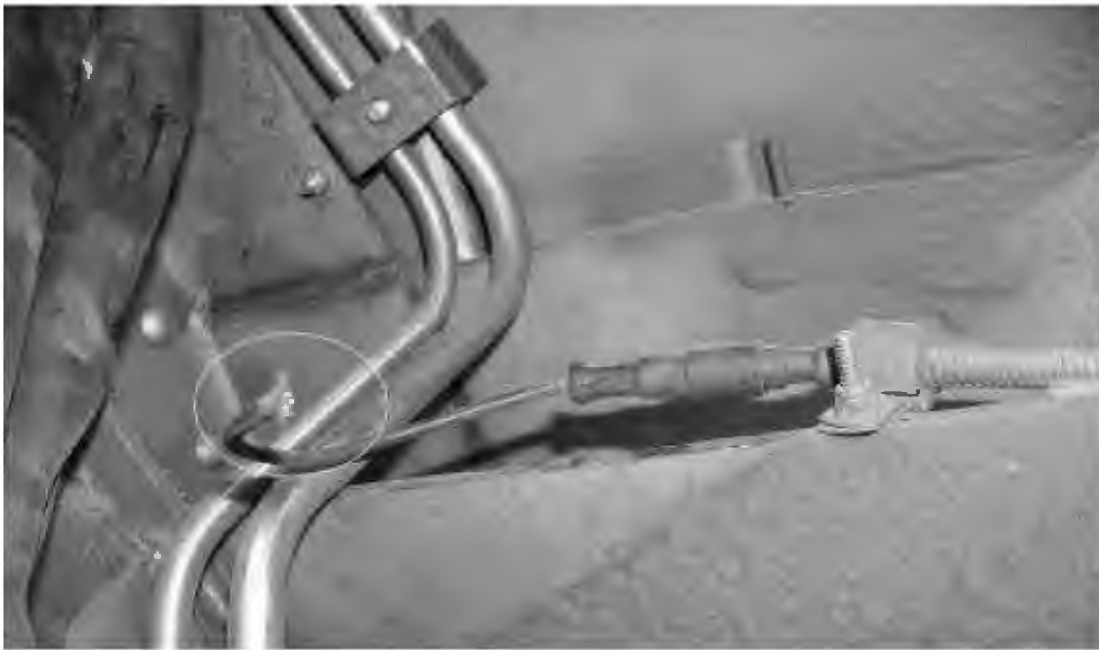
BROKEN LEFT REAR ABS SENSOR (5,451 TEST MILES)
