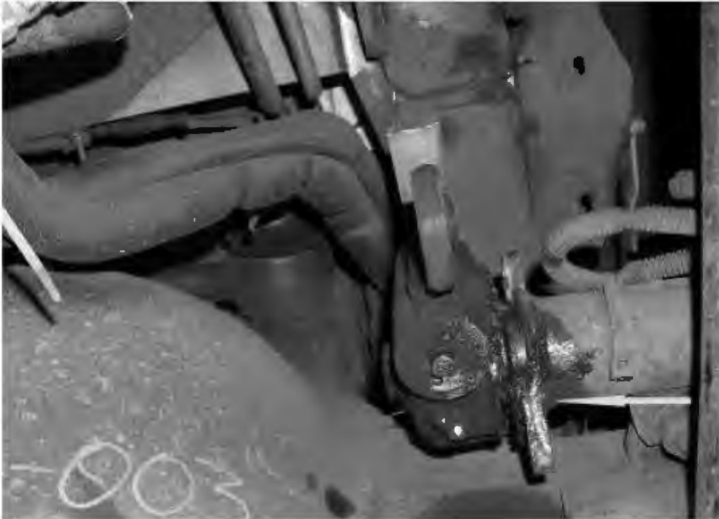
BROKEN RIGHT REAR BRAKE CHAMBER BRACKET (6,516 TEST MILES)
