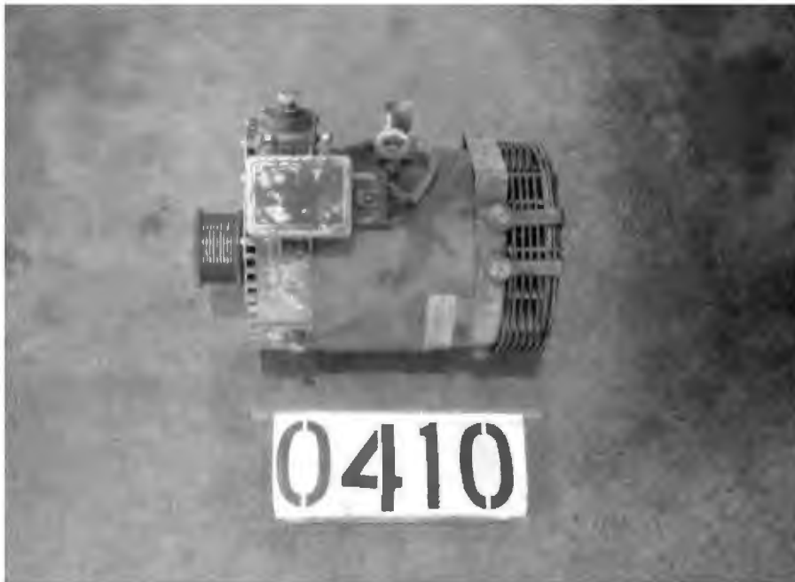
ALTERNATOR REMOVAL AND REPLACEMENT (0.75 MAN HOURS)
