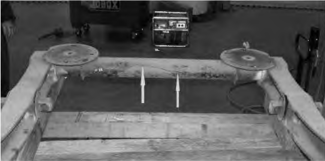
CRACKED TRANSVERSE BAR IN REAR, LOWER CONTROL ARM ASSEMBLY (3,785 TEST MILES)
