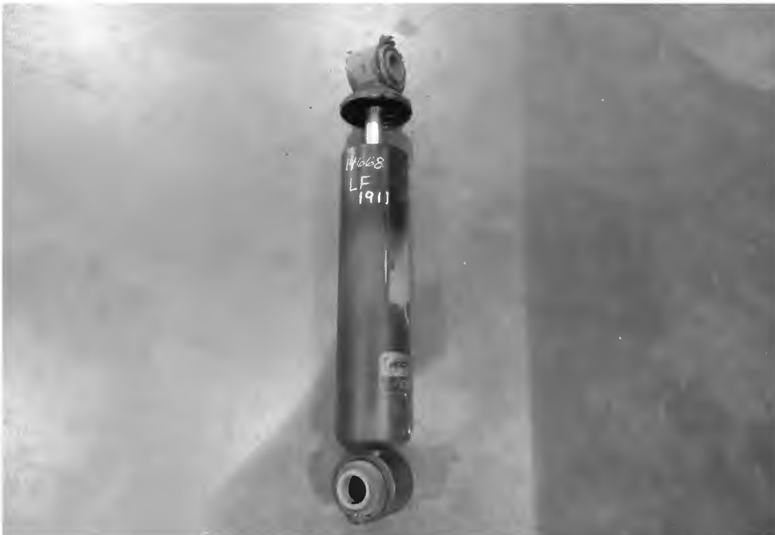
FRONT SHOCK LEAKING (11,491 TEST MILES)
