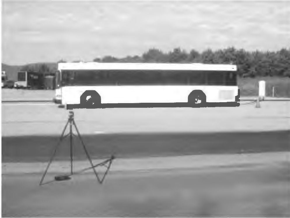
TEST BUS UNDERGOING EXTERIOR NOISE TESTING
