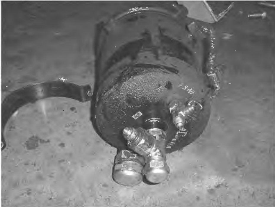
CRACKED HYDRAULIC RESERVOIR (12,487 TEST MILES)
