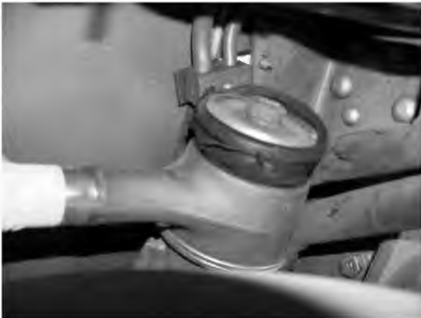
FAILED BUSHING; REAR AXLE LATERAL BAR (6,614 TEST MILES)
