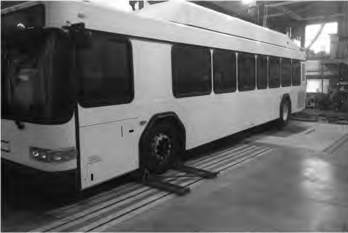
BUS TESTED ON CHASSIS DYNAMOMETER FOR EMISSIONS AND FUEL ECONOMY
