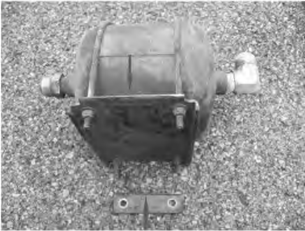
FAILED AIR TANK MOUNTING BRACKET (8,074 TEST MILES)
