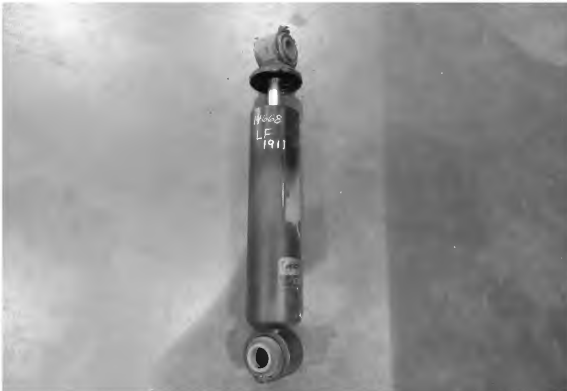
FRONT SHOCK LEAKING (11,491 TEST MILES)
