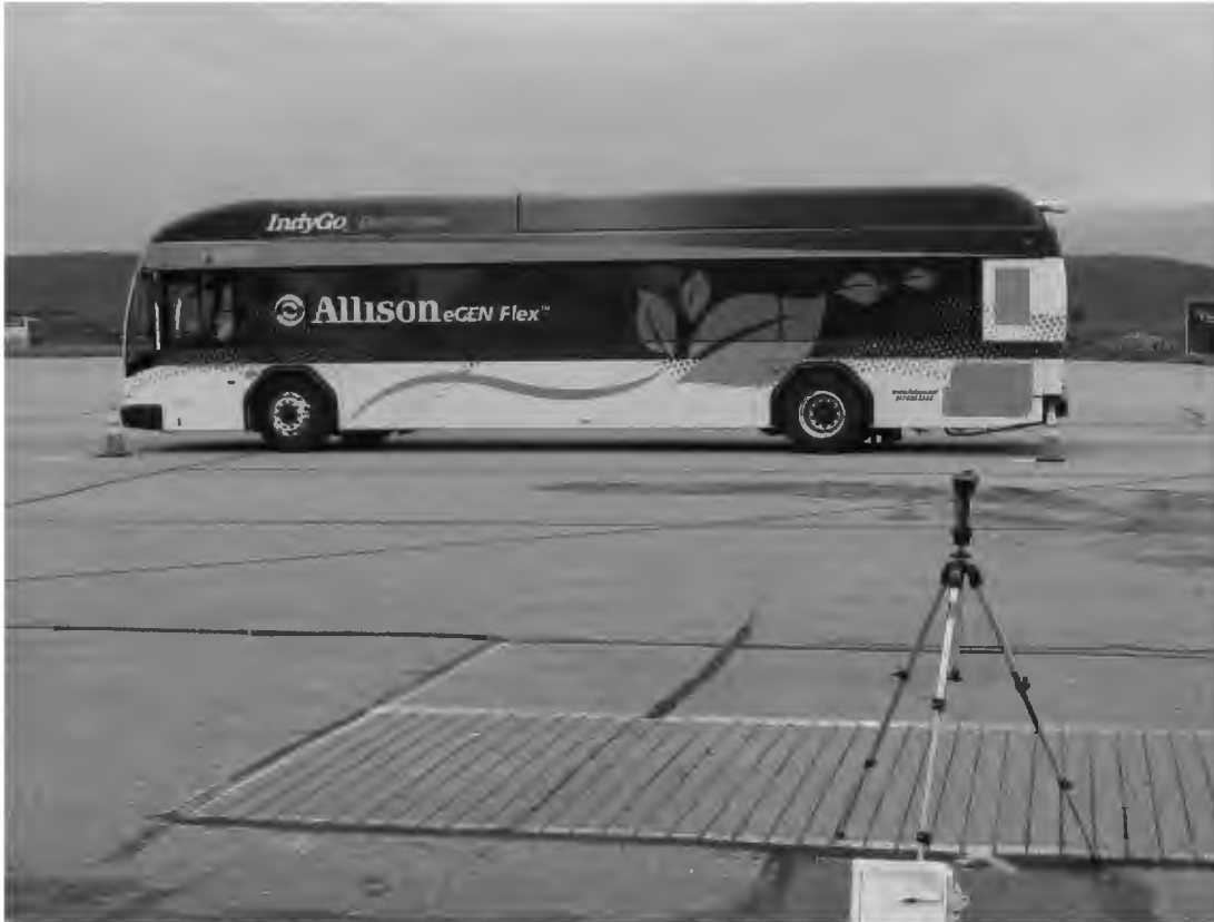
TEST BUS UNDERGOING EXTERIOR NOISE TESTING
