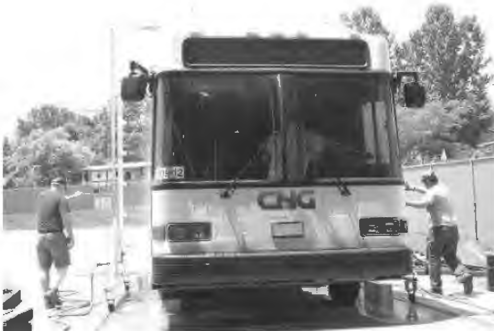
RIGHT FRONT WHEEL SIX INCHES HIGHER
