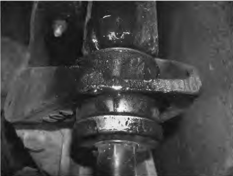
FRONT SHOCK LEAKING OIL (4,379 TEST MILES)
