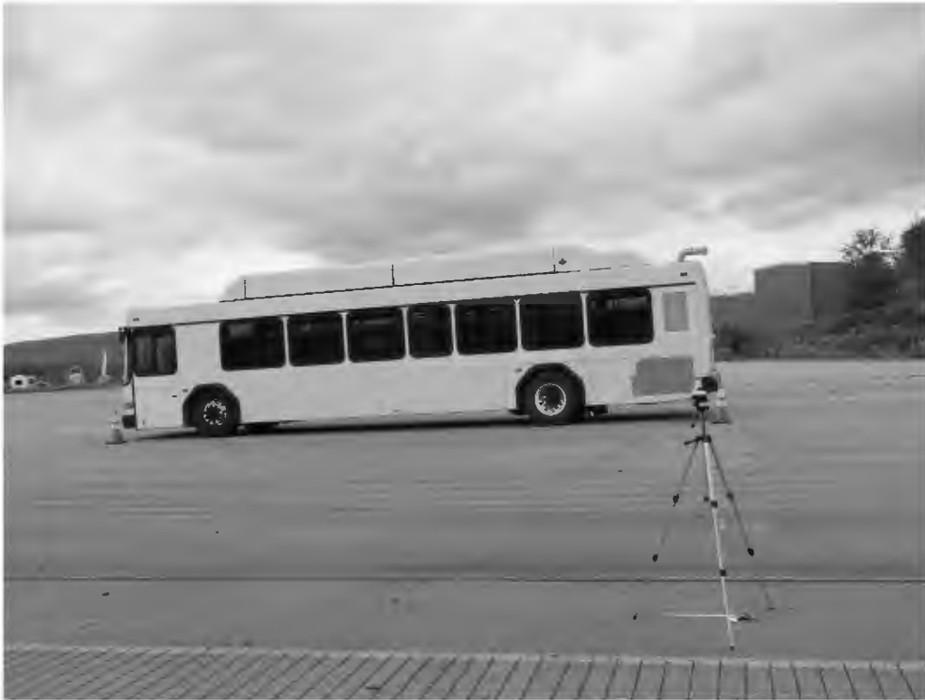
TEST BUS UNDERGOING EXTERIOR NOISE TESTING
