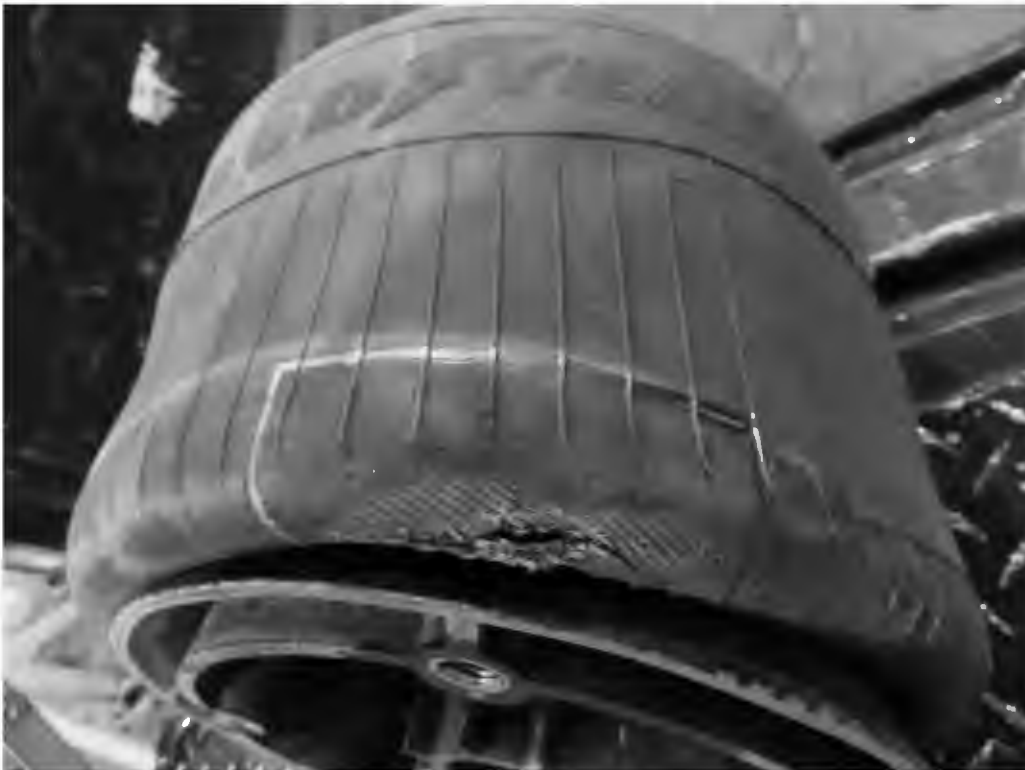
DRIVER'S SIDE FRONT AIR BAG LEAKING (10,976 TEST MILES)
