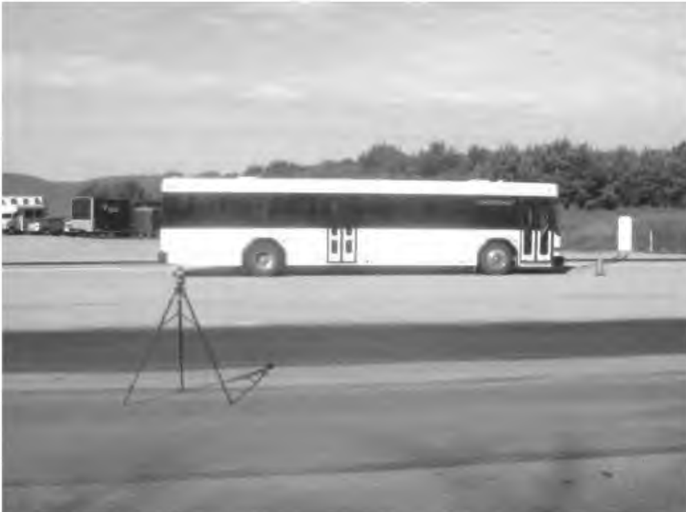
TEST BUS UNDERGOING EXTERIOR NOISE TESTING
