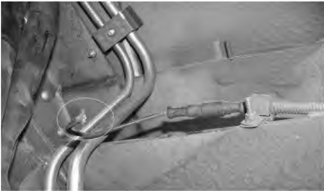
BROKEN LEFT REAR ABS SENSOR (5,451 TEST MILES)
