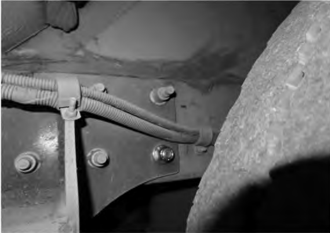
BROKEN HUCK BOLT REPLACED (11,491 TEST MILES)
