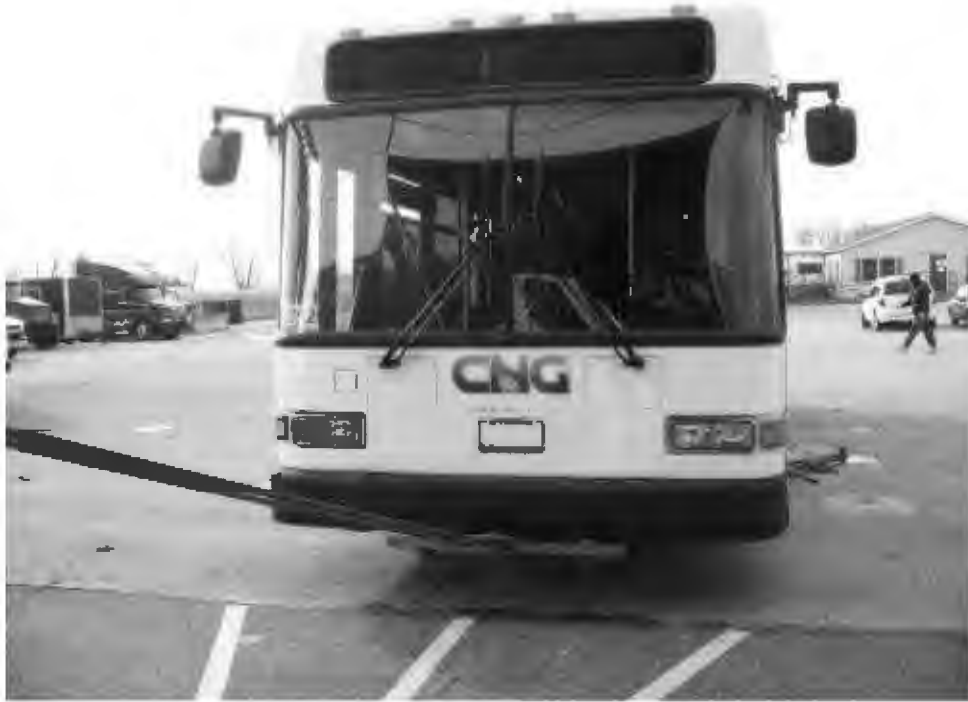
FRONT 20° UPWARD PULL
