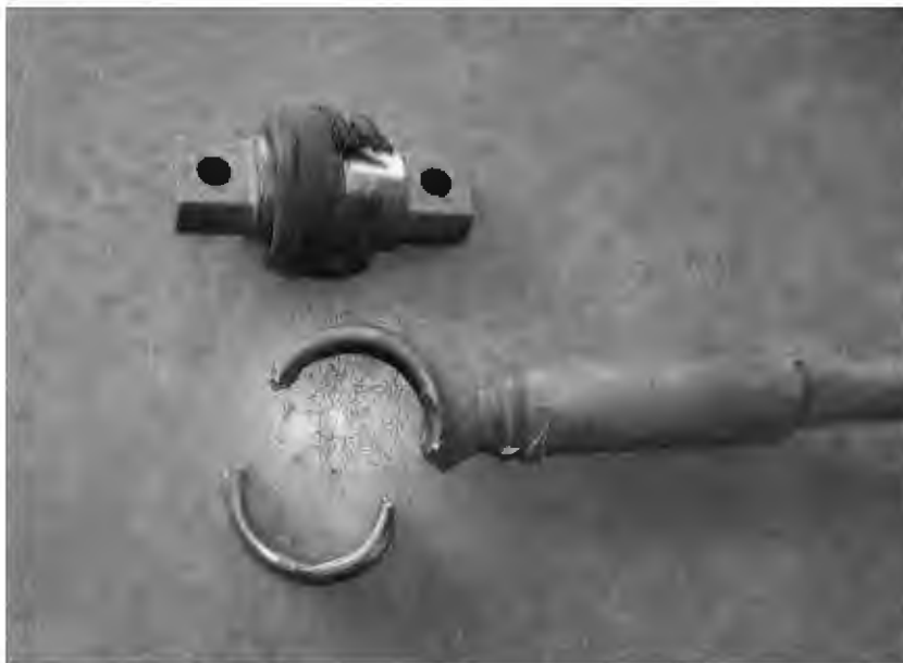
BROKEN TRACK ROD EYE (3,785 TEST MILES)
