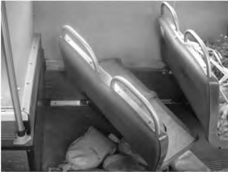
BROKEN SEAT FRAME (5,500 TEST MILES)
