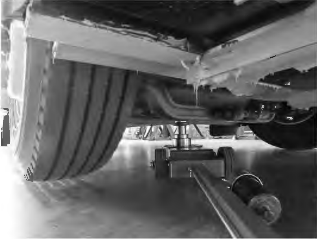
JACK IN PLACE-FRONT
