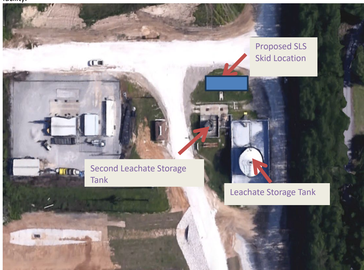
Figure 3-2. Proposed System Location for the ROBOX Unit Adjacent to the Leachate Storage Tank at HCNWLF (Image by Google Earth)
