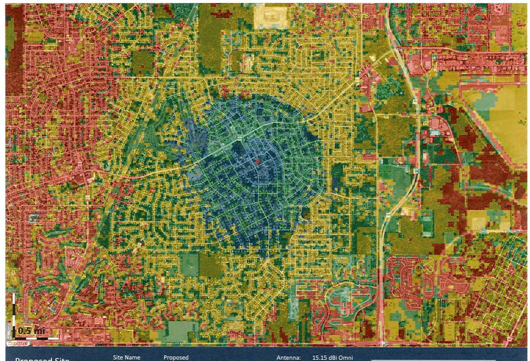
Proposed Site 850 MHz Coverage Site Name Latitude: Longitude: Proposed N28.463244 W82.507883 Antenna: 15
