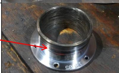
A photograph of a metal flange. A red arrow points to the seal ledge area.                                           |
