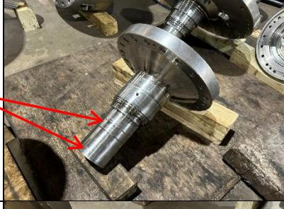
A photograph of a large metal shaft assembly. Two red arrows point to the pulley fits on the side of the shaft.        |
