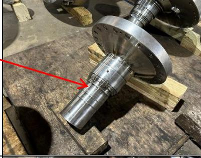
A photograph of a large metal shaft assembly. A red arrow points to the main bearing fit area at the end of the shaft. |
