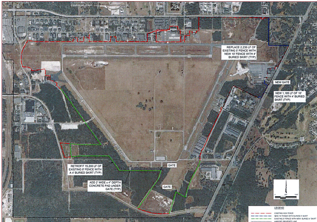
Figure 1 – Security and Wildlife Fencing Layout
